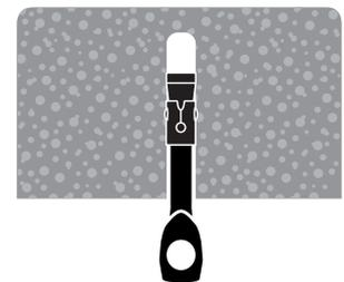
NB: Pull on anchor head with claw hammer to set anchor
