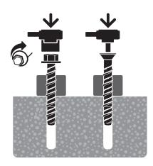
Install with either a socket or cordless impact driver. Apply pressure against the fixing and rotate to engage the first thread. Continue to tighten the anchor until flanged head is firmly seated against fixture.
