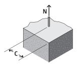
To achieve published tension loads the anchors should be installed at least 8 x the anchor diameter from a concrete edge. If edge distance is closer than 8 x the anchor diameter apply the appropriate reduction factor as outlined in the EDGE DISTANCE TENSION TABLE to the published load to ascertain the reduced load.
