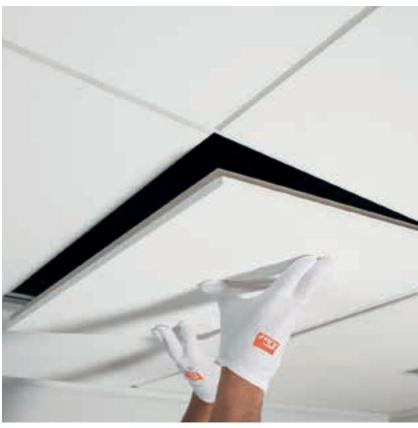
The grid structure of the acoustic ceiling THERMATEX® SF Acoustic is concealed. The special edge detail completely conceals the grid construction, except for a 7 mm wide shadow gap. At the same time, installation remains easy. The tiles are pushed into a conventional grid structure consisting of T24 profiles from below. Thus, the ceiling achieves minimal installation heights (from 75 mm) and is particularly suited for use in refurbishment projects.
