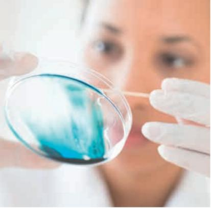
Determination of the resistance to a variety of fungi, bacteria and yeast strains as per ASTM G21/G22.
