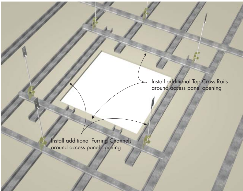
FIGURE 6 Stratopanel Access Panel Framing Perspective
