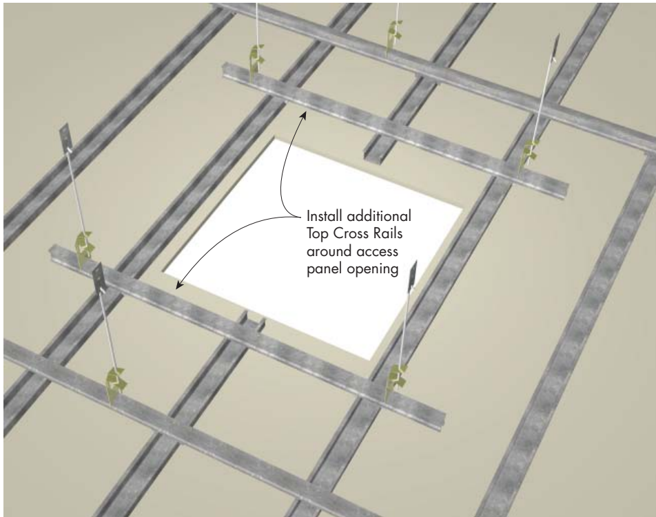
FIGURE 5 Stratopanel Access Panel Framing Perspective
