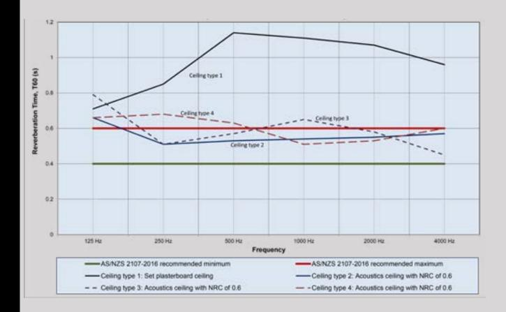
Ceiling type 1 does not meet the reverberation time requirements of AS/NZS 2107-2016.
