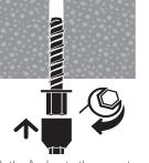
size socket driver and install anchor perpendicular to the base material substrate. Be sure not to over torque the anchor. Install with either a socket or cordless impact driver.
