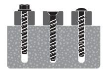
4 Continue to tighten the anchor until flanged head is firmly seated against fixture. Be sure not to over torque the anchor. Installation complete!
