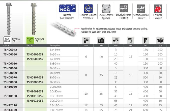
C1 Seismic assessment only valid for the following embedment depths: TSM06 - 40mm + 55mm / TSM08 - 65mm / TSM10 - 85mm / TSM12 - 100mm / TSM14 - 115mm. C2 Seismic assessment only valid for the following embedment depths: TSM08 - 40mm + 65mm / TSM10 - 85mm / TSM12 - 100mm / TSM14 - 115mm
