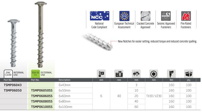
C1 Seismic assessment only valid for the following embedment depths: TSMP06 - 40mm + 55mm
